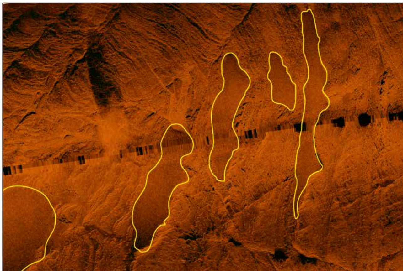
Fig 5.6 Sidescan sonar data with sand areas ringed in yellow.
