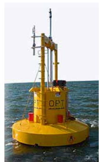
Fig 3.2 An example of point absorber device – Ocean Power Technologies' PowerBuoy ( http://www.oceanpowertechnologies.com/ ).
